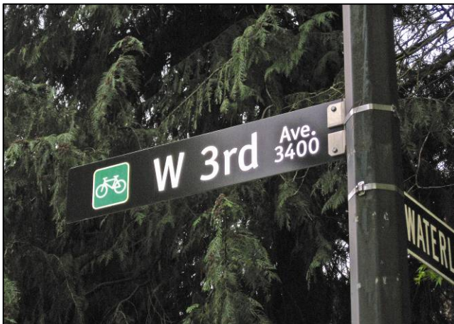
Figure 14: Road name sign using miniature TAC IB-23 bicycle symbol
